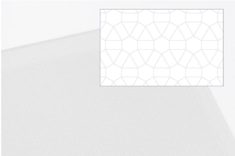
Image 1: With a newly developed, subtle pattern, coated glass can be enhanced by means of laser processing so that high-frequency wireless communication waves can penetrate the surface without attenuation.
