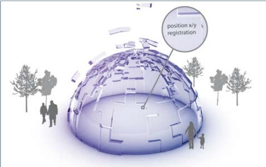
may be helpful to match the single pane with its later position in the facade. In this manner, the architectural freedom allows one to create facades with glass of individual shapes and free forms. Apart from its form, an increasing diversity of properties also results in the need for glass to be tracked and allocated. This
