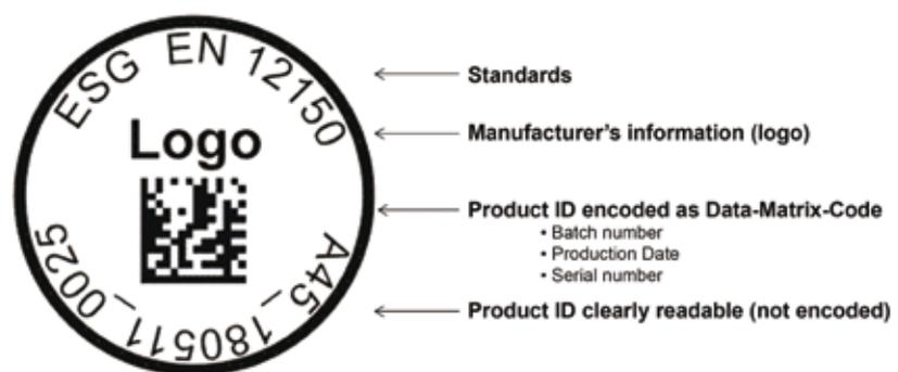
Figure 2: Characteristic marking layout for toughened glass
